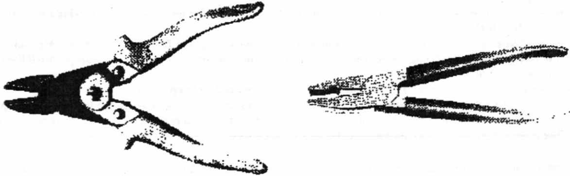
Figures 3-4: Bolt cutting action side cutters and grip/cutter pliers
